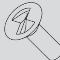
Figura 3.3 – Parafuso "one way"
